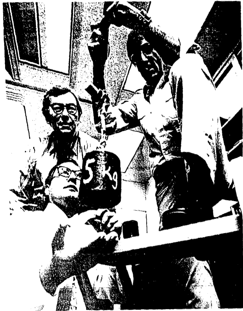
A NEW EXPERIENCE Bell Laboratories scientists (left to right) Hargovind Sarin, Harold Schonhorn and Charles Kurkjian demonstrate the tensile strength of a stronger-than-steel, hair-thin glass fiber using a five kilogram (about 11 pounds) weight. Fabricated at Bell Labs, the new glass fibers have withstood pullings of more than 600,000 pounds per square inch, making them stronger than stainless steel wires of the same diameter.
