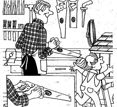
Several handsaws are tools of necessity in any handyman's workshop. Not only can they perform most cutting jobs, but they should do them quickly, easily and accurately. To assure years of performance, wipe the saw after use (inset) with an oily cloth.
